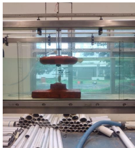
Fig 4: In-channel wave pump model
